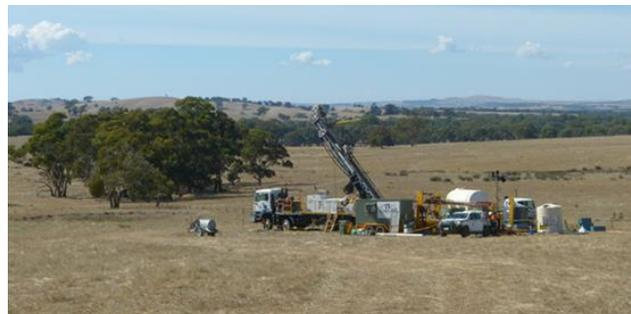
Diamond drilling (like water bore drilling) is one of the most advanced forms of exploration
